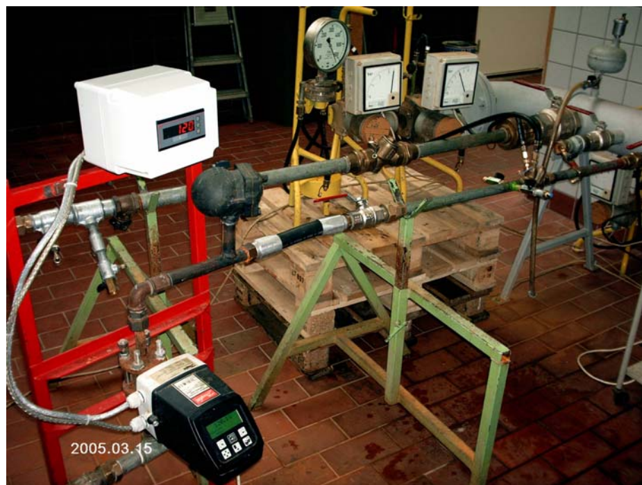
Figure 2 View showing test lengths, flow meter and pressure transducers.
