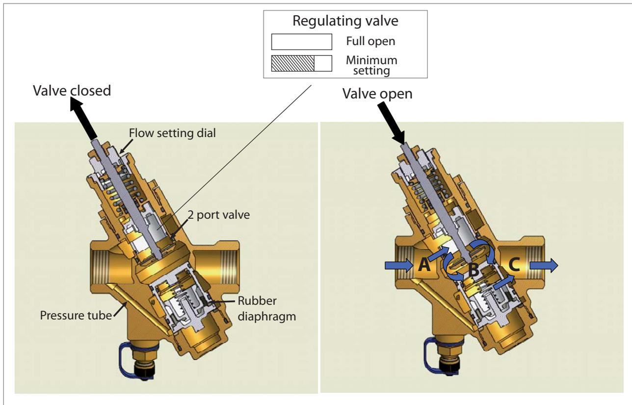
**Figure 5:** Cross section diagram of OPTIMA valve
