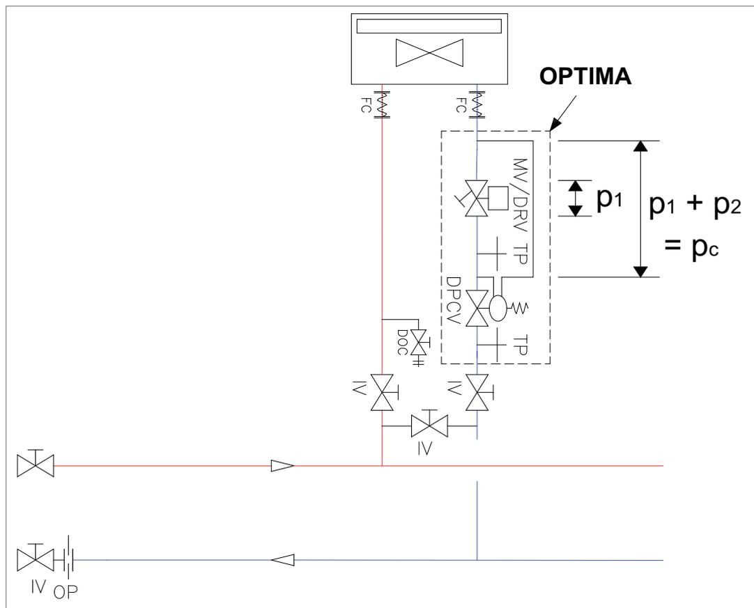
**Figure 4:** Valve authority in terminal branches with Optima valves
