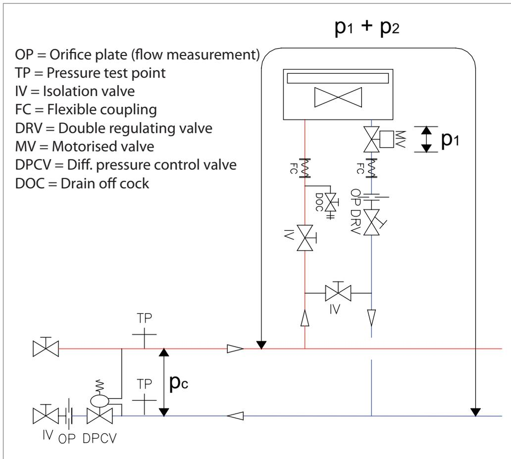
**Figure 2:** Valve authority in terminal branches with individual 2 port
