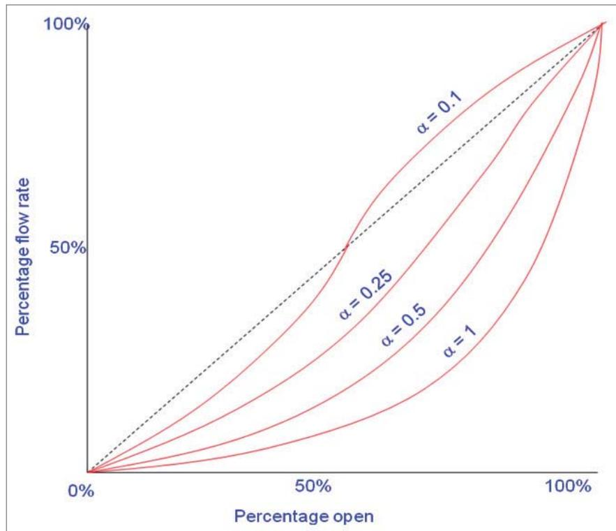
**Figure 3:** Effect of valve authority on an equal percentage valve
